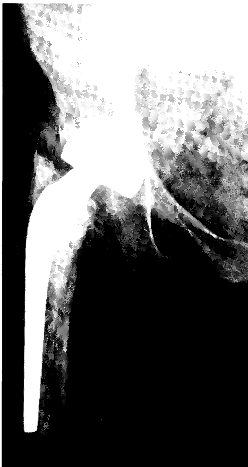
FIG. 1. Roentgenogram shows failed cemented CoCr alloy stem. Varus migration stem with severe osteolysis of lateral cortex.
