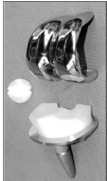
Fig. 11 Photograph of the Self-Aligning-II total knee prosthesis. Note the maintenance of the single axis of curvature for the J-curve of the femoral component, the newer rounded femoral condyles in the medio-lateral plane designed to avoid edge-loading, and the change to a chromium-cobalt tibial baseplate from a titanium tibial baseplate.
